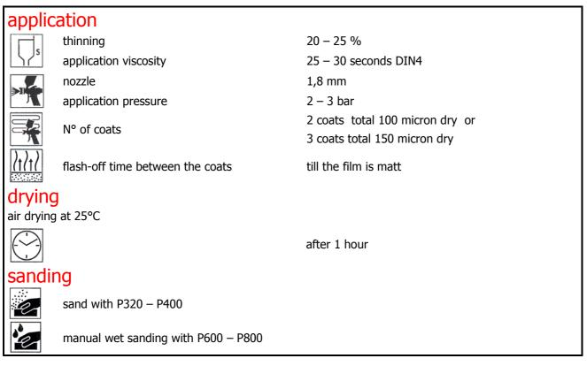
ATTENTION: in case of high thickness applications (3 coats – 150 micron) it is necessary to wait 2 hours at 25°C before sanding
